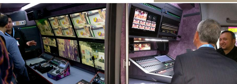
Designed from ground-up to be able to undertake both live and post production requirements. The MINI OBVAN has dedicated separate video and audio production rooms with independent access doors and sound insulation in between.
