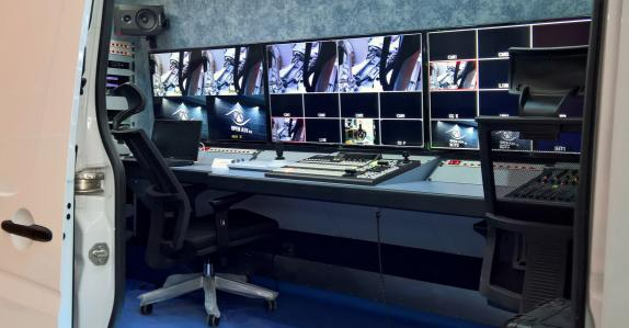
Our classical DSNG design follows the long-established best practices for the uplink vehicles. Our base unit is a panel van with high roof and 5,000 kg load bearing capability. We divide the interior into two by placing the equipment racks directly above the wheels on the back. The area on the back is used for a super silent generator and fixed and portable cable drum storage. When the portable cable drums are removed you can easily access back of the racks.
